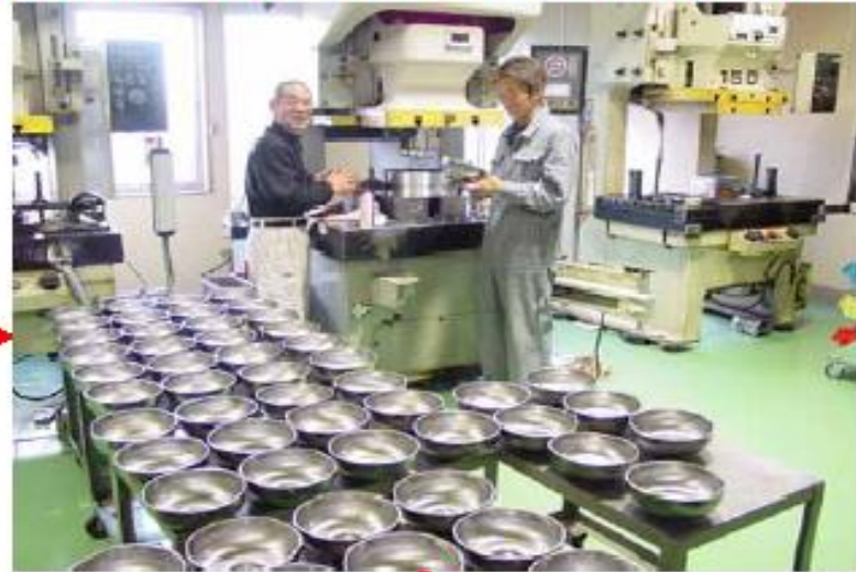
56 half-cells were pressed in a few hours
