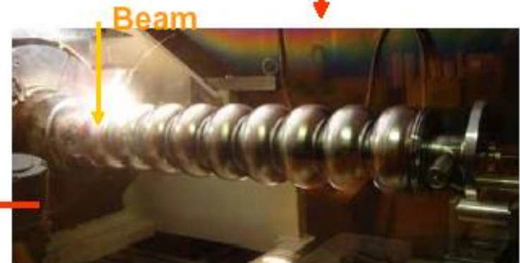
EBW of end-beam-pipes and cell-part
